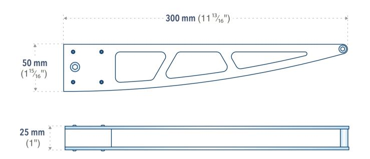
Orientation: Left or Right (Both left and right must be used when using 524 D01 as shelving supports)
