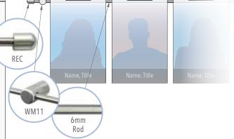
The hook-on holders/sleeves are designed as 1/8" thick clear acrylic folded style frames with a special molded top that can hook onto the 6mm diameter rods. Sleeves are available in both "clear acrylic" or "non-glare acrylic".
