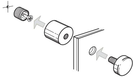
**Three Part Fitting** - Includes M10 Stud-Cap, Standoff Spacer/Barrel and Coupling Anchor.
